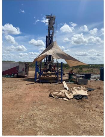
Figure 4. UDR1200 drilling on RDD019, EPM 17968, Clermont
