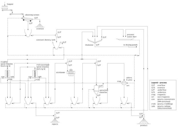
Figure 4 – block flow diagram "BFD" of the overall process
