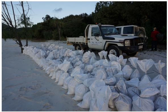
**Figure 3:** Sample bags with white sand collected from drilling during the July/August 2020 Cape Flattery drill program
