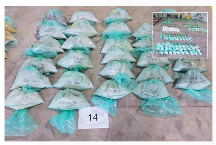
Figure 6 - Sand samples from December drilling programme at IHC Robbins in preparation for Metallurgical testwork to commence
