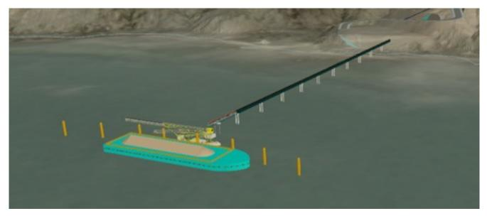
The stacker will be a vendor package like the one shown in Figure 7.5 with its own MCC to operate the equipment and barge load head-end conveyor motor.
