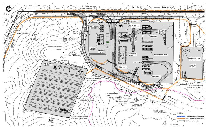
Figure 7.3: Mine industrial area general arrangement
