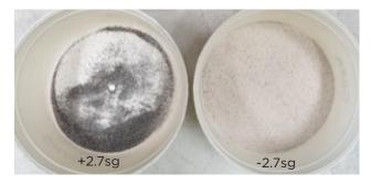
A sub-sample of the float fraction was treated in a high-energy attritioning cell to clean the surfaces of the sand particles. The residence time was five minutes with an operating solids density of ~75% w/w. The attritioned sample was wet-screened at 106 $\mu$ m to remove any liberated slimes. The assay for the attritioned and deslimed product is shown in Table 6.4.
