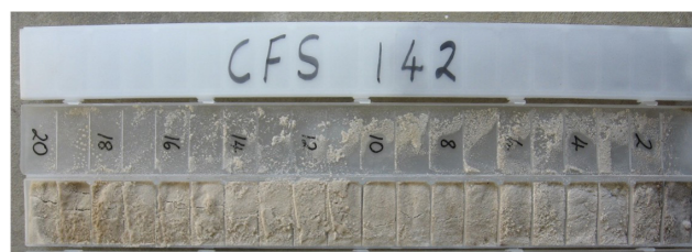
Figure 3: Chip tray samples from hole C142 (being 36m in depth)
