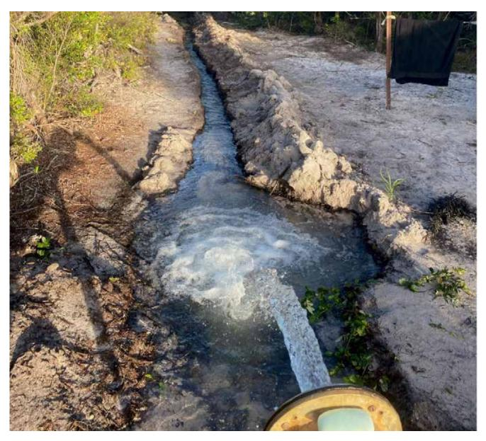
Figure 4: Water bore pump out test
