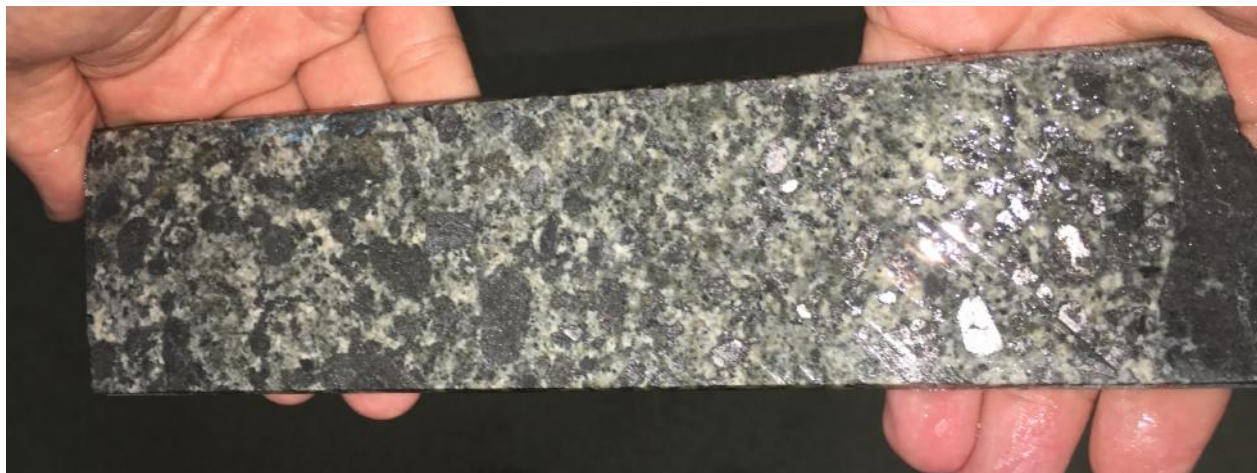
Figure 2: The darker areas above illustrate the frequency, density and consistent distribution of the graphite mineralisation associated with other darker alteration minerals through the core of WD001. The high graphite bearing blebs typically show high metallic reflectance in certain light angles
