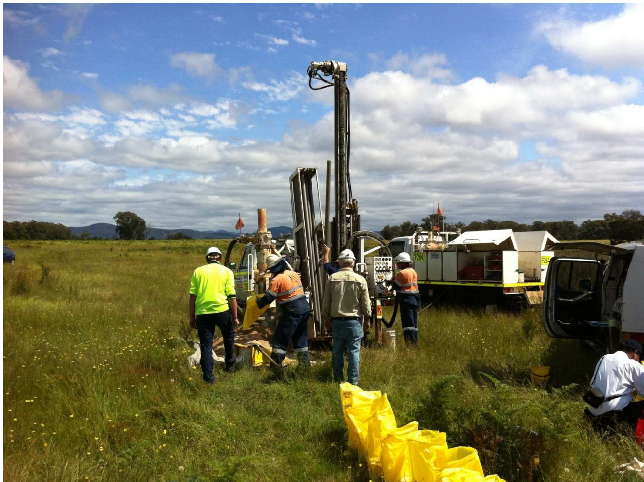
Figure 3: Low impact aircore drilling in the central portion of the Glenaladale area (December 2011)
