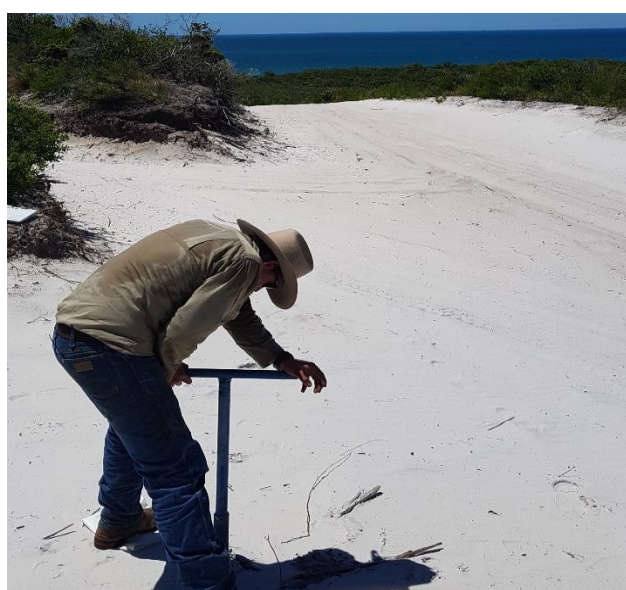
Figure 3 – Process of taking an Auger Sample
