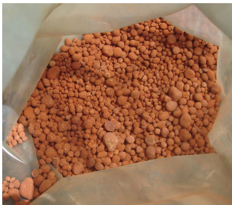
Figure 1. Pisolitic bauxite from aircore drilling at Wenlock.
