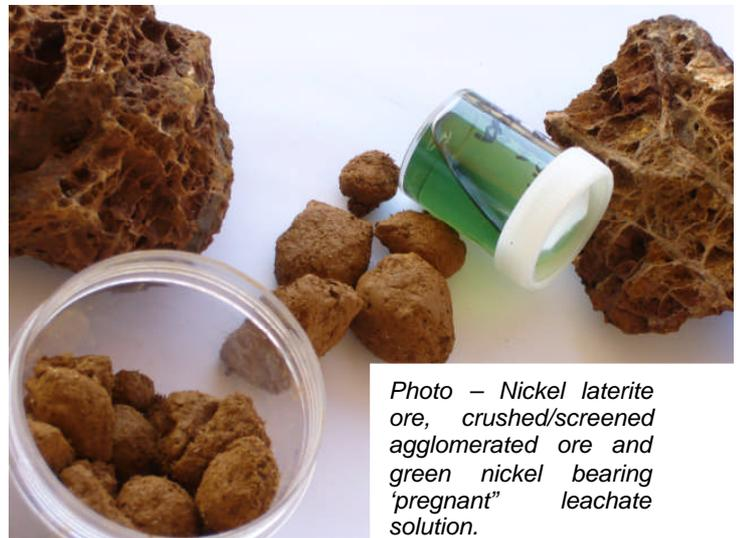
Photo – Nickel laterite ore, crushed/screened agglomerated ore and green nickel bearing 'pregnant' leachate solution.
