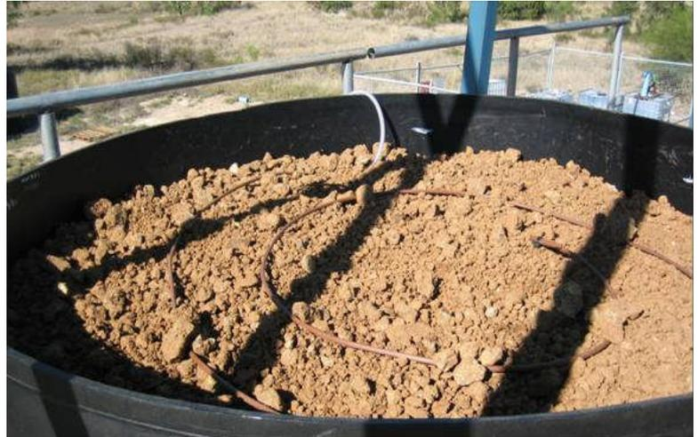
Photo – Top of loaded large leaching column (4m high by 1.6m diameter) with agglomerated nickel laterite ore.
