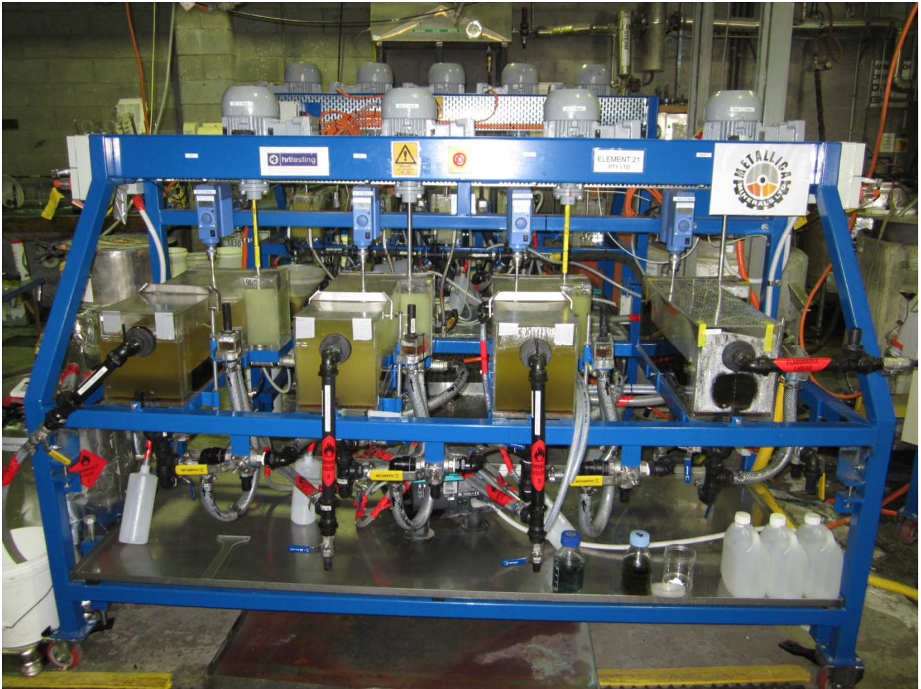
Figure 1. Metallica Minerals' purpose built pilot plant located in Brisbane for scandium extraction and recovery from scandium rich pregnant liquor solutions (PLS) generated from the SGS Lakefield Oretest high pressure acid leach (HPAL) pilot plant (in Perth) treating NORNICO scandium rich nickel laterite ore types.
