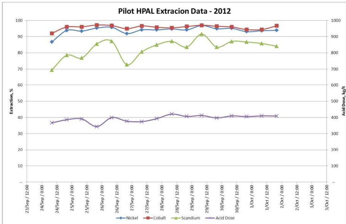
Figure 1: Sc-Co-Ni Metal Extraction (LHS) & Acid Consumption (RHS)
